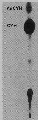
Figure 1. Tlc autoradiogram showing the degradation of 14 C-CYH 3 days after application to the surface of an orange
